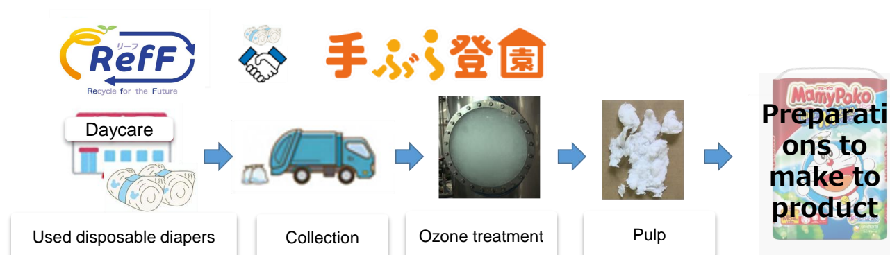
Process flow recycling from collecting used diapers from daycare facilities to creating new product
